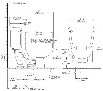
THIS COMBINATION IS DESIGNED TO ROUGH-IN AT A MINIMUM DI-MENSION OF 305MM (12") FROM FINISHED WALL TO C/L OF OUTLET. \* DIMENSION SHOWN FOR LOCATION OF SUPPLY IS SUGGESTED. SUPPLY NOT INCLUDED WITH FIXTURE AND MUST BE ORDERED SEPARATELY
